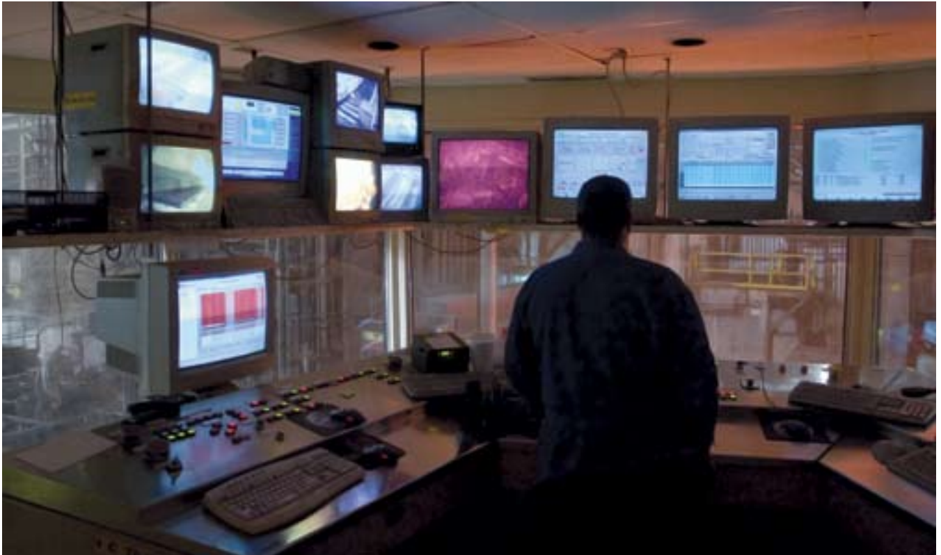
The loneliness of the automated workplace: From a sound-proofed and air-conditioned “pulpit,” a solitary worker controls the operation of a steel-plate rolling mill. A dozen video monitors and computer displays keep him company. The use of computer control in manufacturing and in other industries has yielded remarkable gains in productivity: We produce more with less labor. And yet, contrary to early expectations, the total number of people employed and the hours they work have not been falling. The photograph below shows the process going on just outside the control pulpit: A slab of glowing steel, enveloped in clouds of steam, is rolled into a thinner plate. No workers are needed near the machinery. The photographs were made at the Nucor Steel plate mill in Hertford County, North Carolina. (Photographs by Brian Hayes.)
